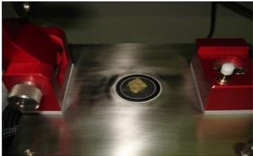
Comb foundation sample prepared for the acquisition of its IR spectrum
